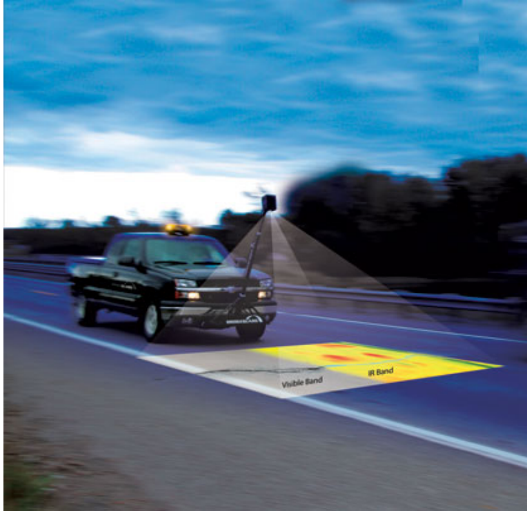
Figure 2-18 Vehicle-mounted infrared thermography scanning (Ruohonen 2013).
