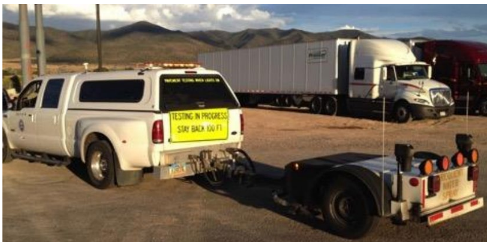
Figure 2-29 Locked-wheel trailer test apparatus (Smith 2016).
