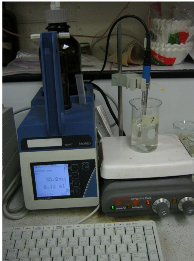
Figure 2-3 Chloride concentration testing.
