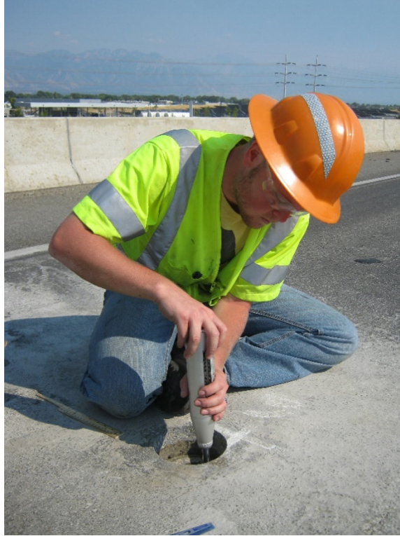
Figure 3-20 Schmidt rebound hammer testing.
