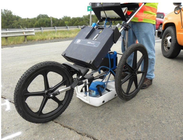
Figure 2-10 GPR testing of a bridge deck.
