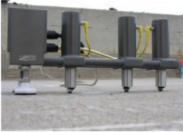
Figure 2-31 Ultrasonic surface wave equipment (Gucunski et al. 2013).
