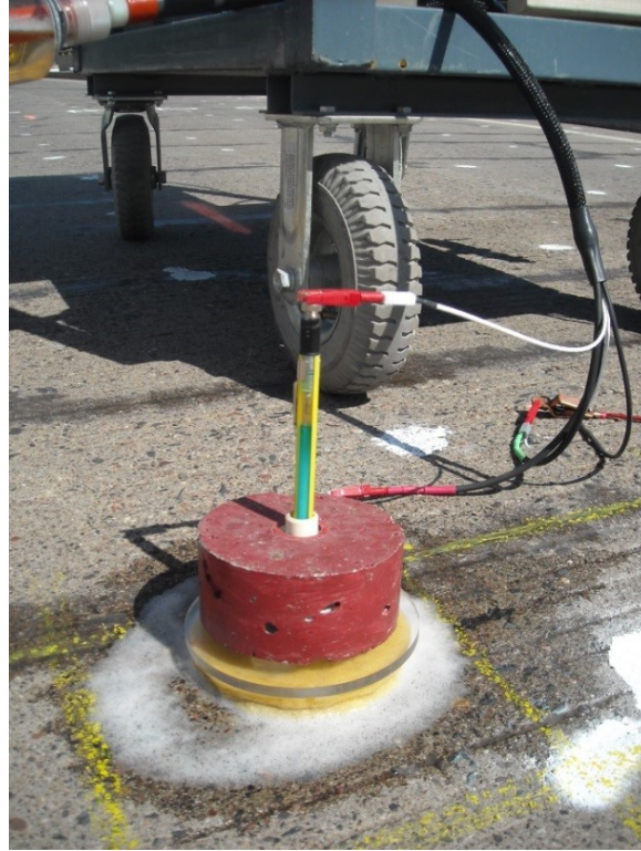
Figure 2-20 Linear polarization testing.
