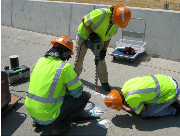
Figure 2-2 Concrete powder sampling for chloride concentration testing.
