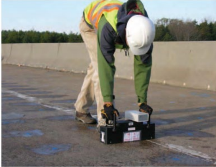
Figure 2-30 Ultrasonic pulse echo testing (Hema et al. 2004).
