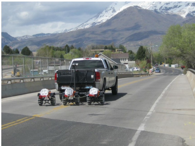
Figure 2-16 Tire-based multi-channel impact-echo scanner.
