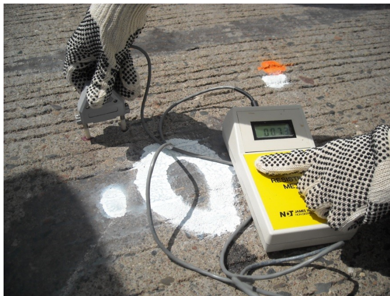
Figure 2-24 Two-prong resistivity testing.
