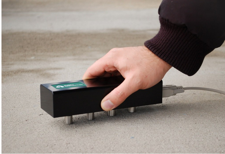
Figure 2-25 Four-prong resistivity testing (Giatec 2013).
