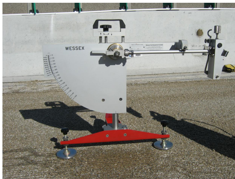
Figure 2-28 Skid resistance testing using the BPT apparatus.
