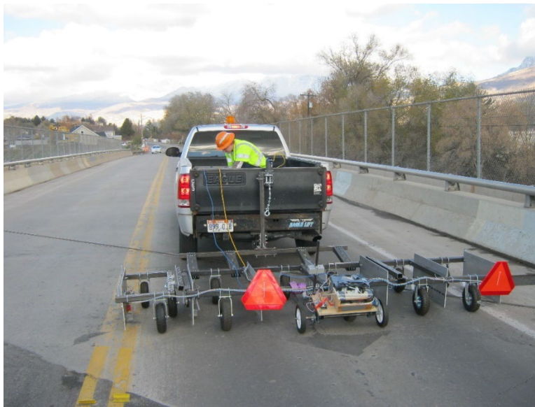
Figure 2-15 Mallet-based multi-channel impact-echo scanner.
