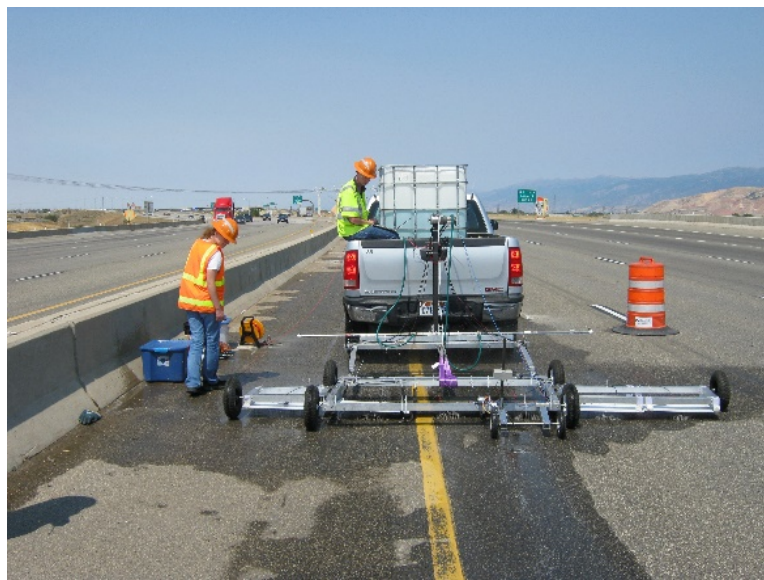
Figure 2-32 VEI testing apparatus (Barton et al. 2019a).
